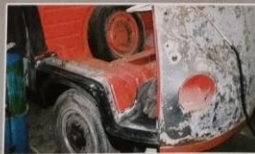
The new panels needed included a pair of cab steps - but doesn't every right hand drive bus?
