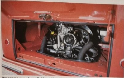
The engine is a nice reliable 1600cc unit, built by VW Speed Shop in Manchester, detailed to perfection and converted to 12 volts
